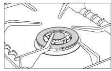
The Wok burner is designed to provide even heat over a large area. It is ideal for large pans and stir frying. When using large pans ensure that the pan does not over hang the edge of the cooktop. For heating smaller pans the smaller burners may be more efficient.
